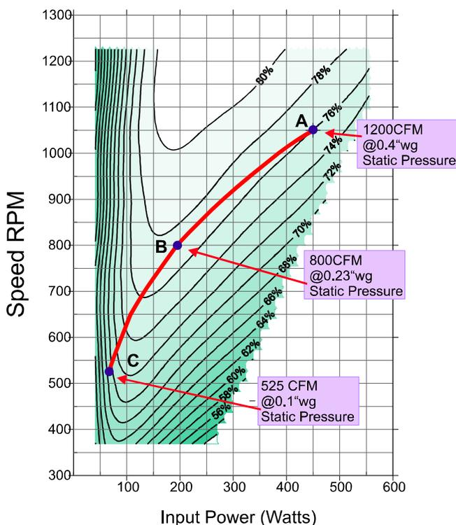
Since dc motors are synchronous machines, the ECM rotor does not slip to change the speed of the rotor. The efficiency of dc motors and the ECM is higher than induction motor efficiency because there are no losses in the rotor – speed and torque can be easily changed in a dc motor by adjusting the voltage and current delivered to the motor, maintaining maximum efficiency over a wide operating range.
